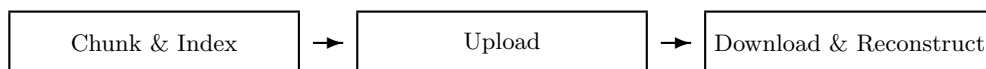
FIGURE 6.1: The experiments aim to optimize Syncany’s core phases in terms of deduplication ratio, processing time and bandwidth consumption. The main focus is on the chunking and indexing phase.
